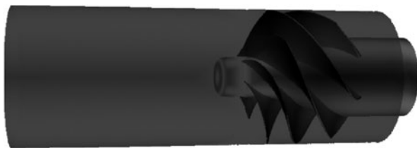
Fig. 7.3 Rocketdyne inducer geometry used for validating computational procedure
